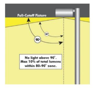
*Full cutoff fixtures do not allow any light to be emitted above the fixture. The fixture controls glare by limiting the light output at 10 degrees below the horizontal.*
